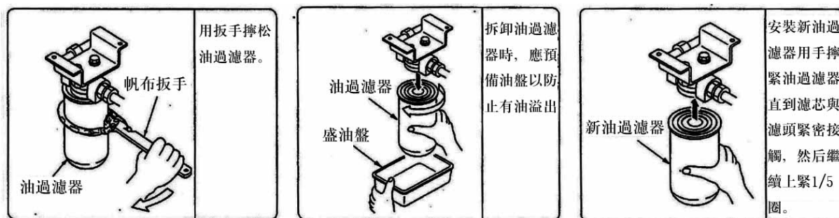
Fig. 5-2 schematic diagram of oil filter replacement
